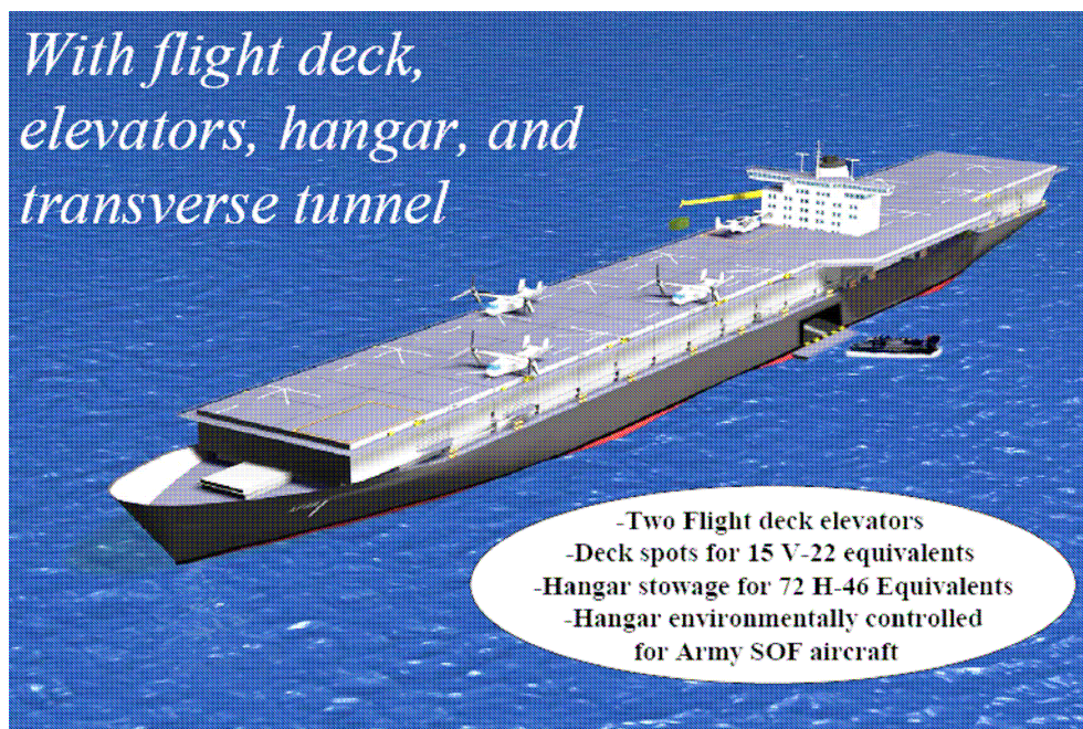
Figure 7 – Maersk S-Class Conversion Concept Design
