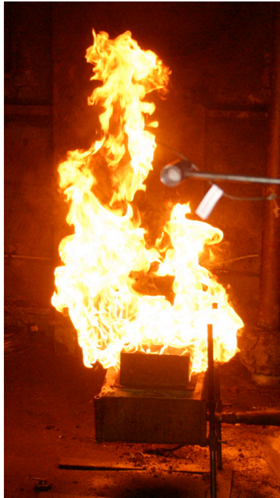
Figure 6. Series 1 Heptane Pool Calibration Fire
