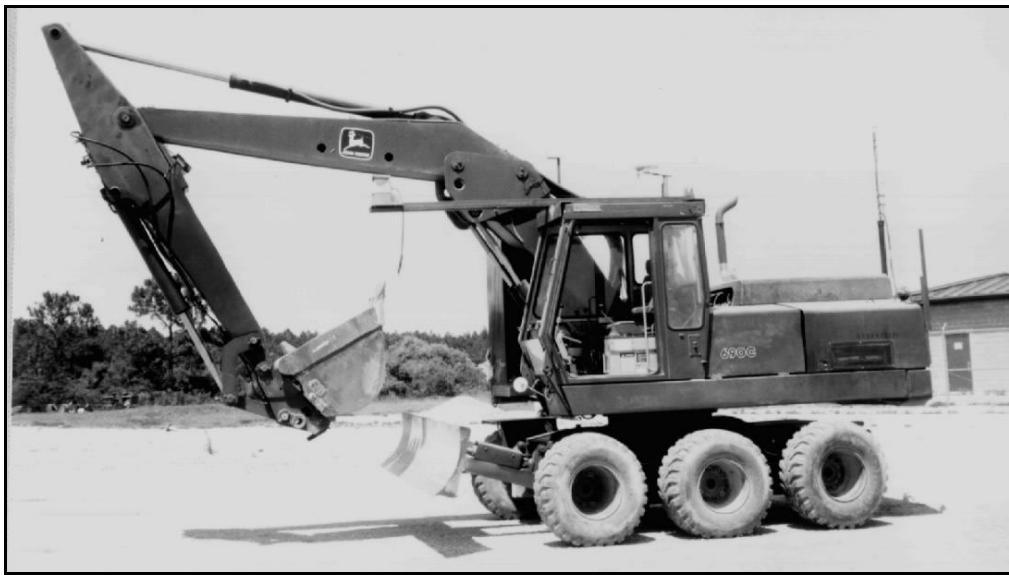
Figure 1-3: The Automated John Deere Excavator
