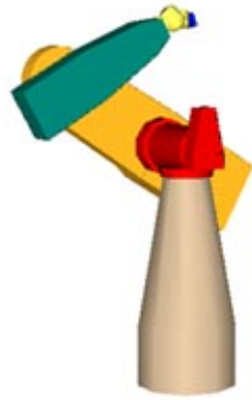
Figure 2-6. Forearm interior singularity of Puma 762 robot
