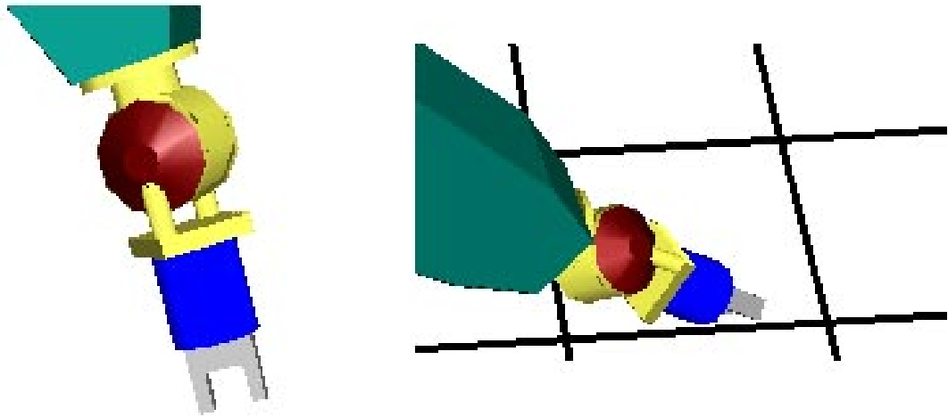
Figure 2-4. Wrist singularity of Puma 762 robot
