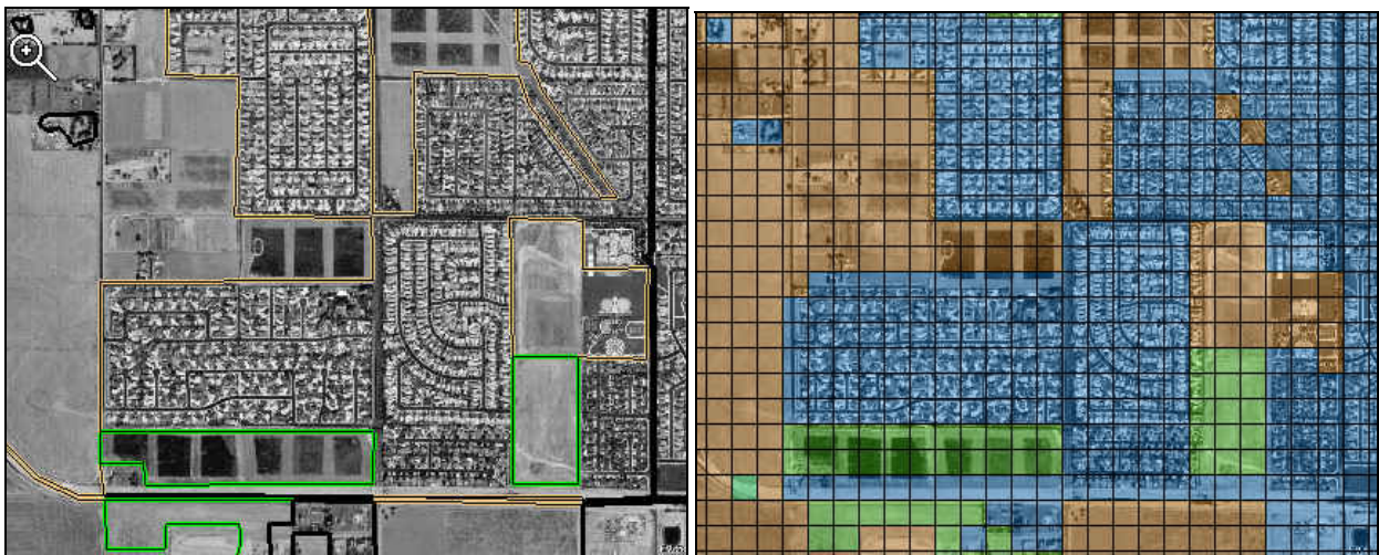
Figure 4. A comparison of the land use GIS data (on the left) with the gridded representation of the land use data (on the right.) The grid is at a 75-m resolution.
