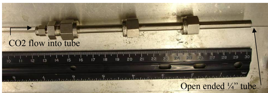
Figure 7: Shroud CO2 injector
