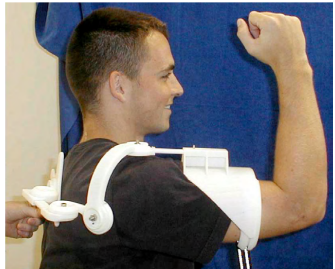
Fig. 5. Side view of Prototype I with elbow and shoulder at 90^\circ flexion.
