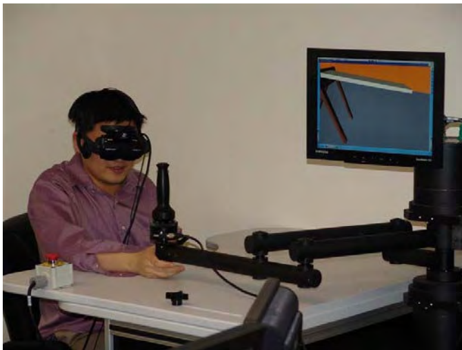
Fig. 2. Subject performs virtual beam task while donning 3D Pro I-Glasses. The vantage angle is changed by using output from an InterTrax2 head tracker mounted on the brow of the display.
