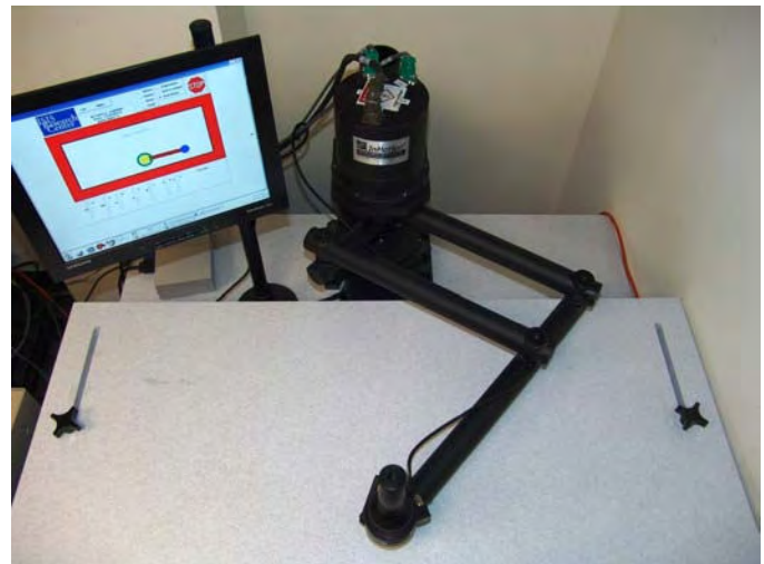
Fig. 1. Top view of InMotion 2 workstation showing four-bar linkage, direct drive motors, workstation, and flat panel display.
