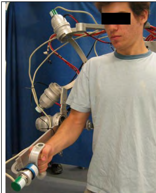
Figure 12: Exoskeleton prototype being test fitted on human subject.
