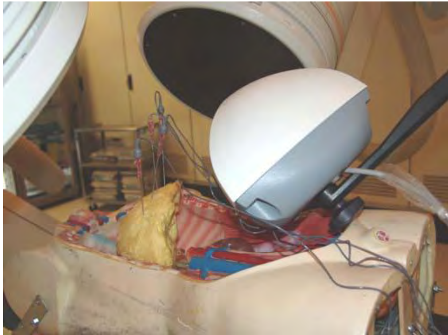
Figure 7: Electromagnetic tracking study in biplane fluoroscopy suite showing both fluoroscopes, dummy torso and moving liver, electromagnetically tracked needles embedded in liver, and electromagnetic field generator
