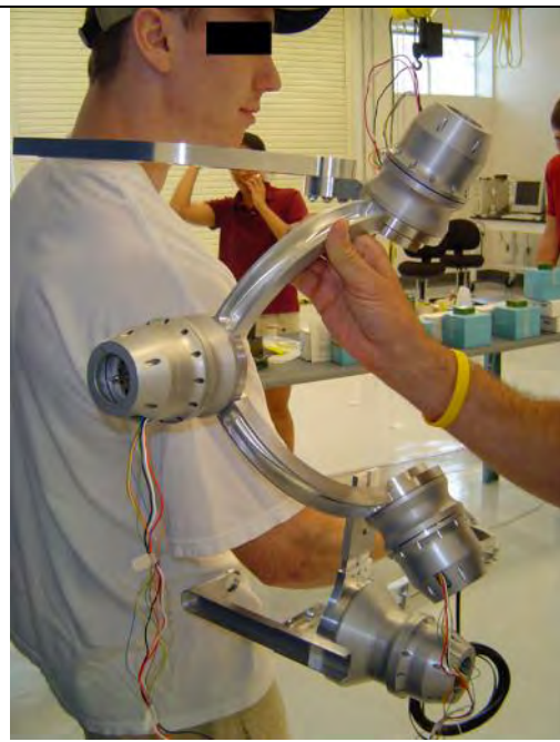
Figure 13: Close-up of the exoskeleton shoulder rotation assembly.
