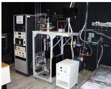
1.5 KW Diamond Deposition System
