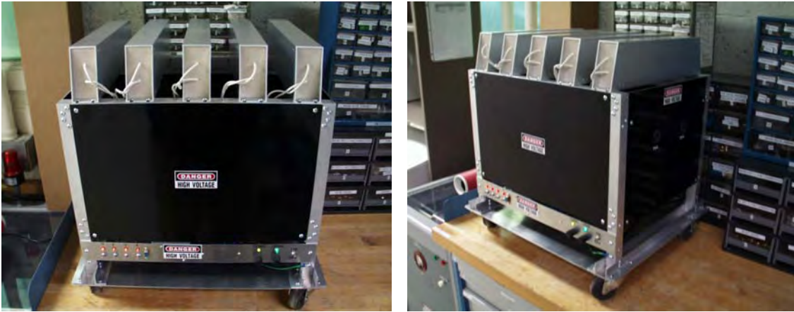
DC-DC Converter Load Bank
