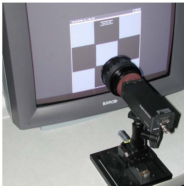
FIG. 1. High-quality CCD camera mounted on custom gantry for measurement of display characteristics. The gantry was capable of both coarse and fine linear movement.
