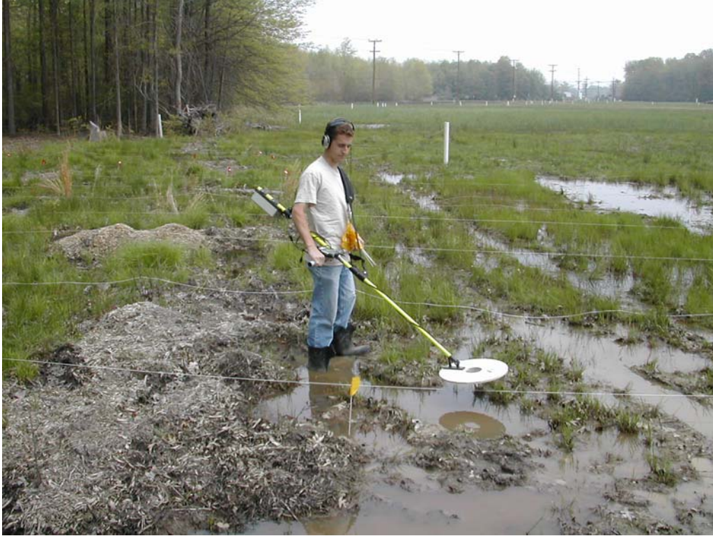
Figure IV-6. Geopex hand-held GEM3 type sensor at APG. This photo illustrates the tendency of the Open Field edge nearest to the Wooded Challenge Area to flood.
