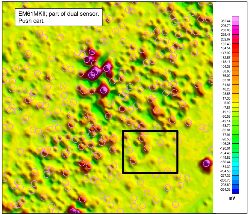
Figure V-1. BlackHawk EMI noise. Within the 9 m × 7 m box, the signal ranged from -40 mV to 80 mV, with a mean and standard deviation of -5 mV and 15 mV, respectively.
