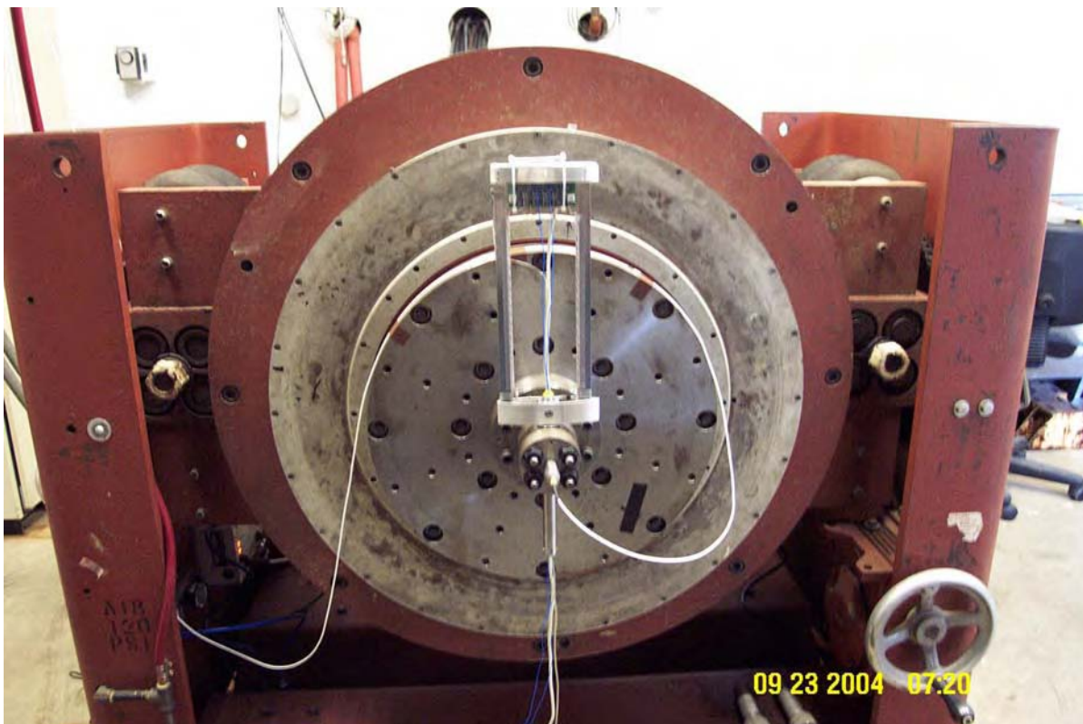
Figure 26. Flex-Wing Skeleton on Shaker Table
