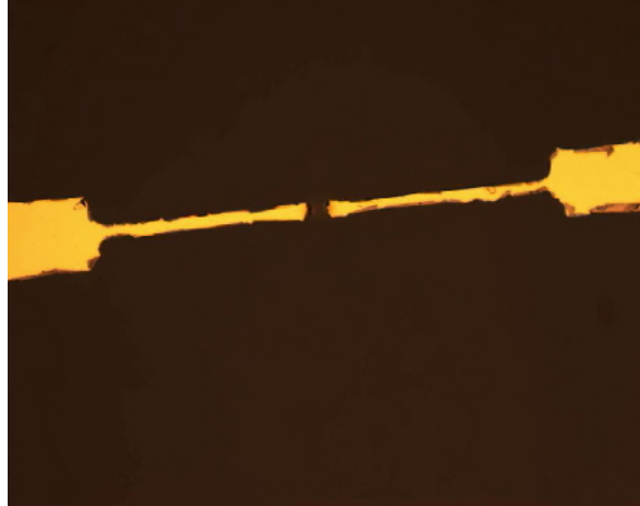
Figure 4.5 This figure shows the results of a Titanium and Gold seed layer patterned with an SU-8 lift-off process. Rough edges around all of the electrode parts can be seen. The rough edges widen the electrode gap by approximately half of a micron.
