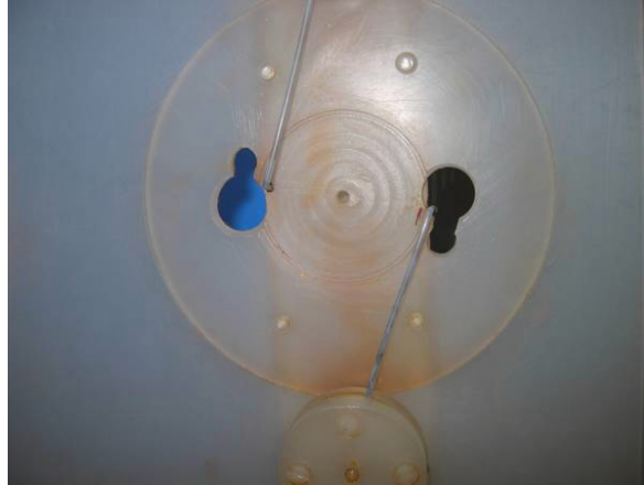
Figure 4.7 This figure shows the contact board used to hold 2 inch wafers and to connect to the seed layers. The two metal contacts shown are held in contact with the seed layer by spring force.
