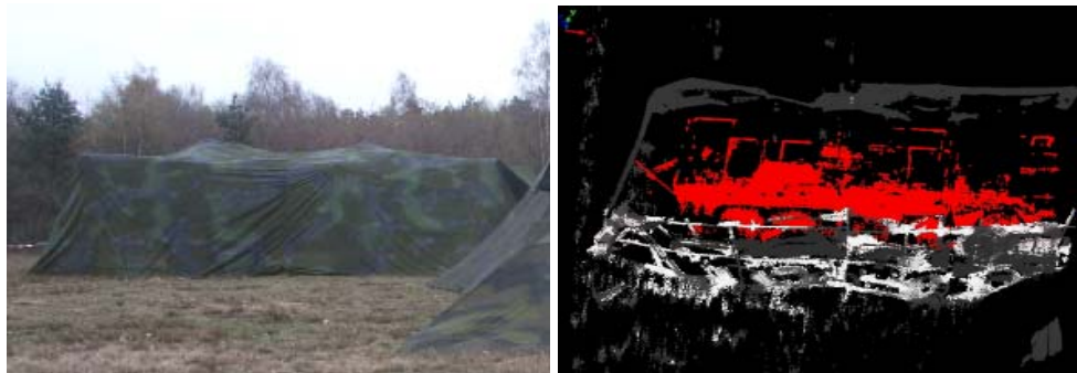
Figure 5. To the left is a photo of a camouflage net. In the corresponding 3-D laser radar image to the right the point cloud has been rotated so that it is viewed from an elevated angle, revealing a truck underneath (highlighted in red for clarity).
