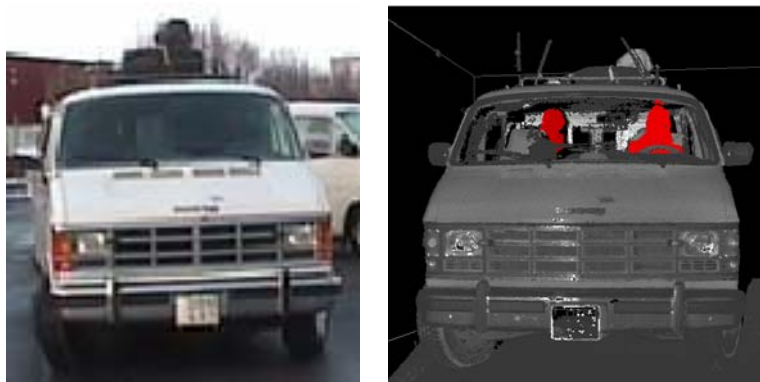
Figure 14. To the left a visual photo and to the right a laser radar image of two people in a van. The drivers face is covered with a bandanna and a passenger (mannequin) is sitting in the rear seat.
