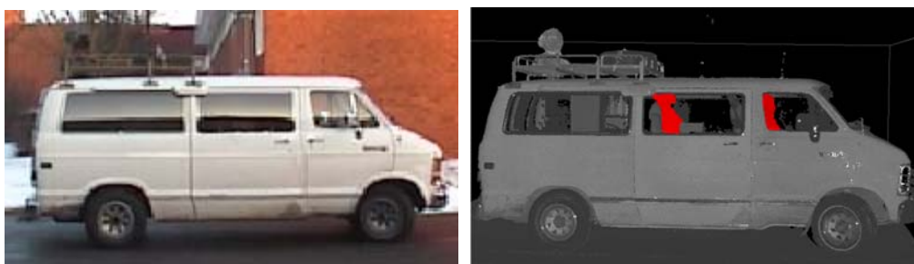
Figure 15. To the left a visual photo of a van. Reflexes in combination with shaded windows makes it difficult to see what is inside the van with a passive sensor. In the laser radar image to the right, both passenger and driver are clearly visible (highlighted in red for clarity).
