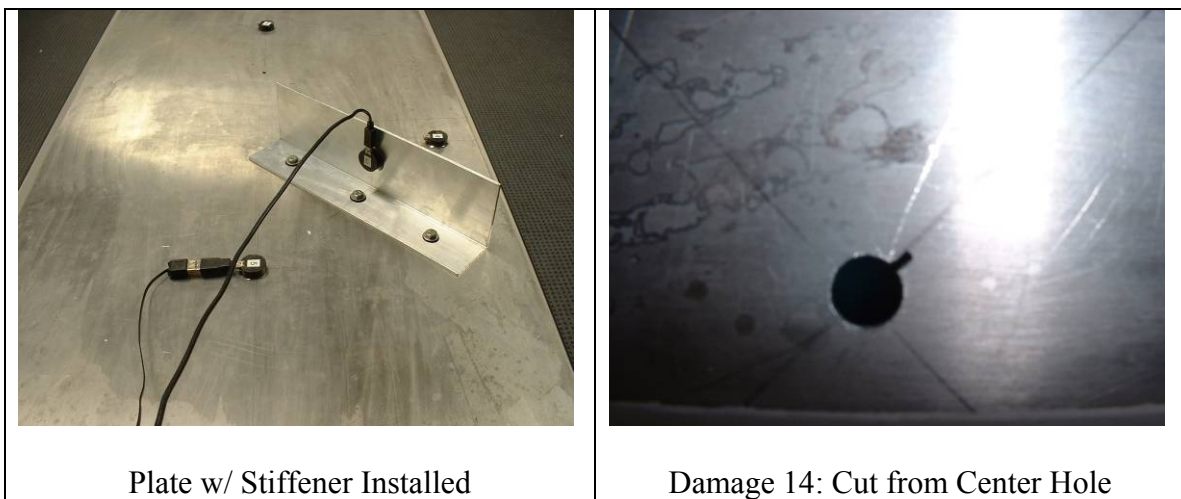
Figure 4.12: Damage Testing w/ Stiffener Installed
