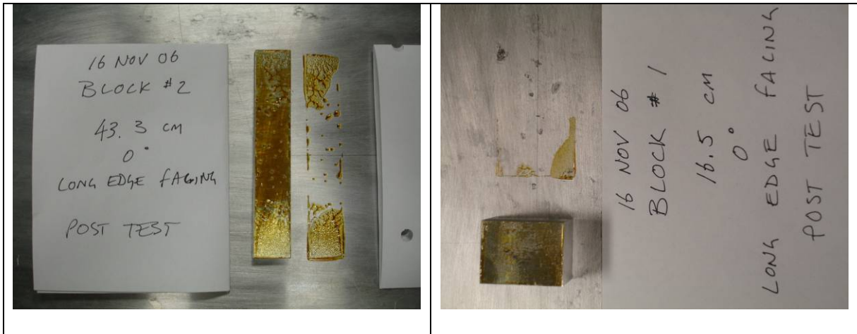
Figure 4.6: Post-Test Pictures Showing Partial Contact of Damage Blocks
