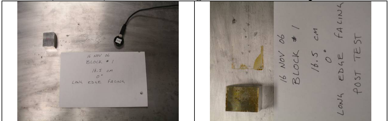
Pulse-Echo (Sensor 0072): 16 Nov 06, Block 1 @ 165mm and 0°, No Damage Baseline
