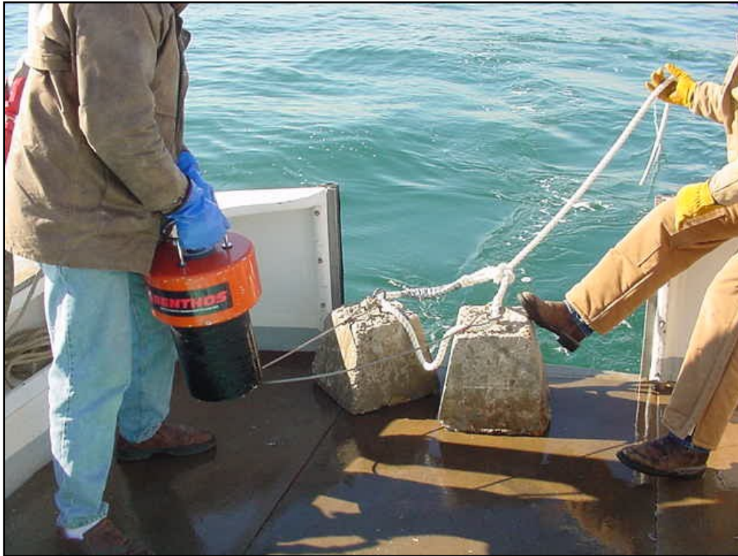
Figure 9. Deployment of pop-up buoy attached to mooring near seaward end of navigation channel.
