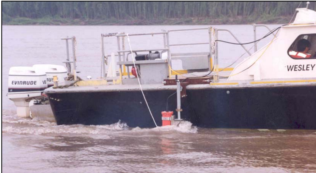
Figure 6. Typical mounting for current transect ADCP on side of survey vessel.
