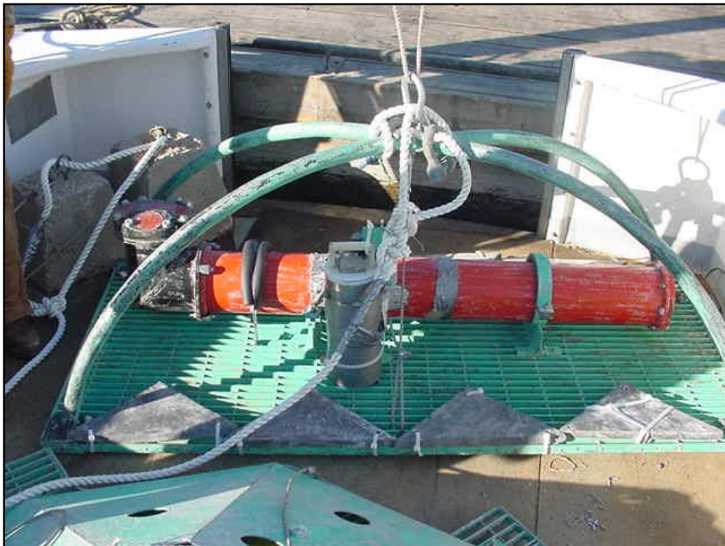
Figure 4. RDI ADCP and water-level gage mounted in mooring frame that was deployed near seaward end of navigation channel.
