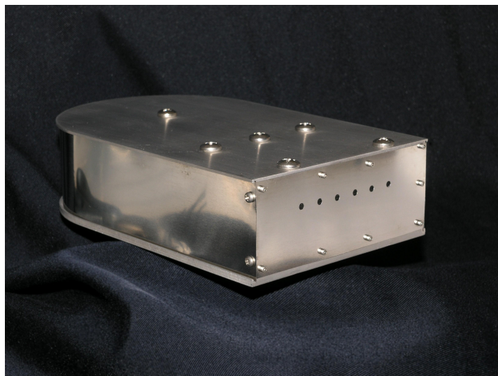
Figure 4. The msLPT is about to undergo final acceptance tests. Six diode lasers drive a special ablation fuel tape behind the output ports. These are fired in matched pairs to maintain a fixed center of thrust. A ns-pulse version is being developed.
