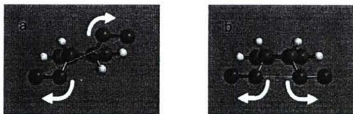
Figure 2.3. The difference between the efficiency of stress activation between trans and cis benzocyclobutene has been attributed to effective torque. a) In trans -benzocyclobutenes, elongational stress applied along the red vector induces a conrotatory motion of the substituents to yield an E,E- o QDM intermediate. b) In cis -benzocyclobutenes, elongational stress applied along the red vector induces a disrotatory motion of the substituents, leading to an E,E- o QDM intermediate.
