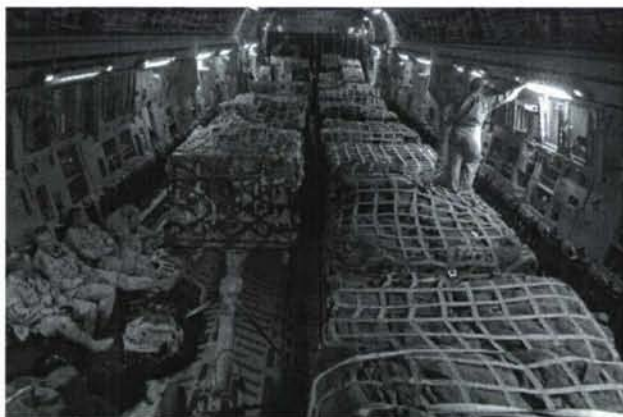
Figure 2-6: C-17 Double Row Pallet Configuration
