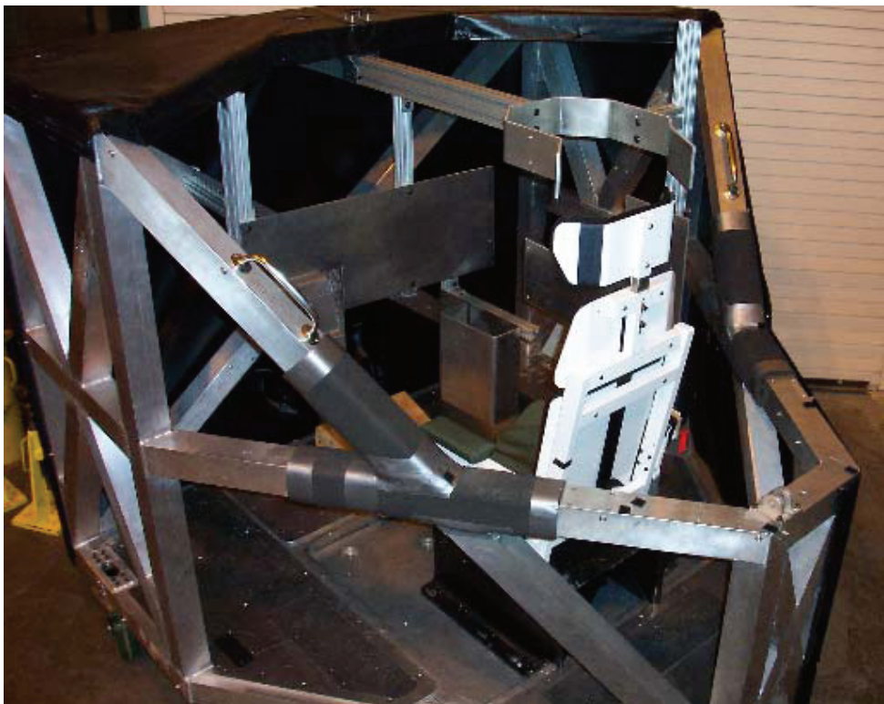
Figure 1. Interior of the RMS, including the aluminum brackets simulating the potential impact points for the head, arms, and legs.
