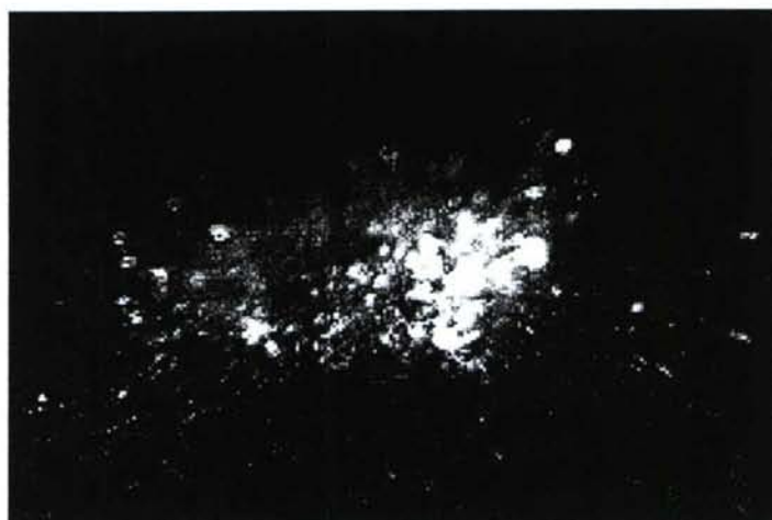
Figure 4.14 Interaction between the spray droplets and the ITO pedestal heated surface at 1000 frames per second (fps) at a flow rate of 5.4 GPH and heat flux of 17 \text{ W/cm}^2 .
