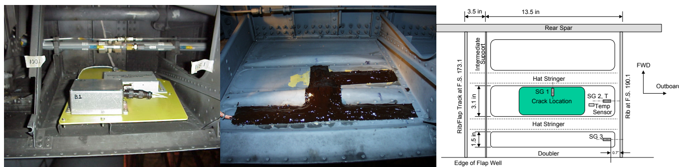
Figure 3. Damage Dosimeter Installation in C-130 as shown by Ikegami, et.al. (2001)
