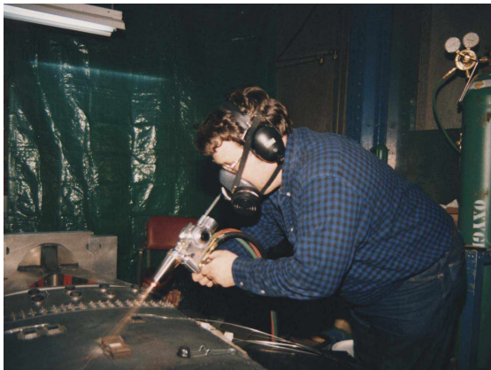
Figure 14: Future Tests Will Use Flame Spray Attachment Technique
