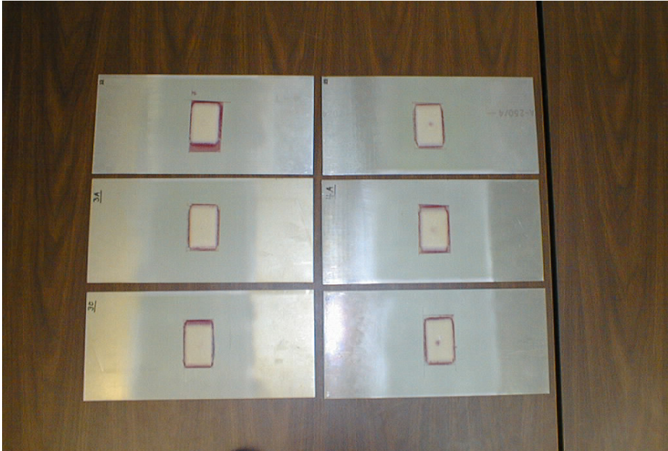
Figure 4b. Large Size (360x170 mm) Test Specimens with Repair Patches
