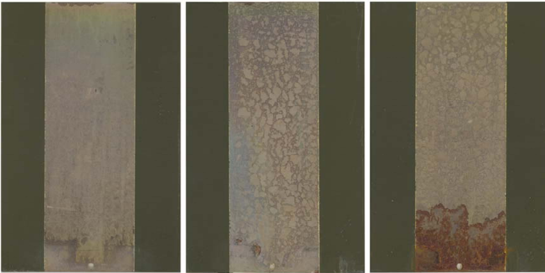
Figure 23. Nucleation of corrosion to lower areas of panels from specimen racks used in GM 9540P.
