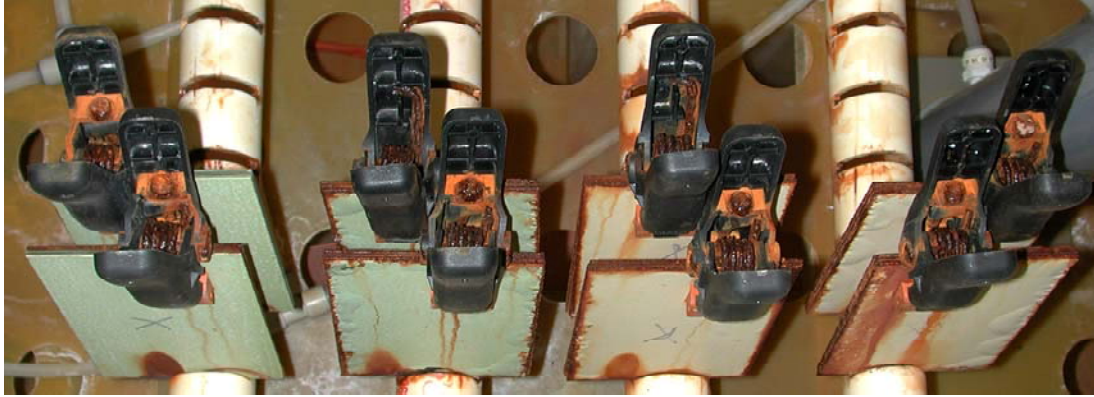
Figure 22. Clamped, unscribed crevice assemblies at 80 cycles of GM 9540P showing relative damage among coating systems 1–4 (from left to right).
