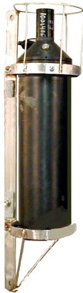
Fig. 4. A PAL in deployment cage. PALs are robust, passive, relatively inexpensive, autonomous, and smart.
