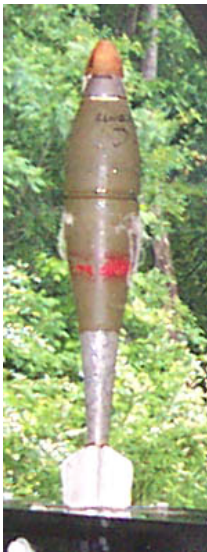
Figure 9. The 81mm mortar round measured on the ERDC test stand.
