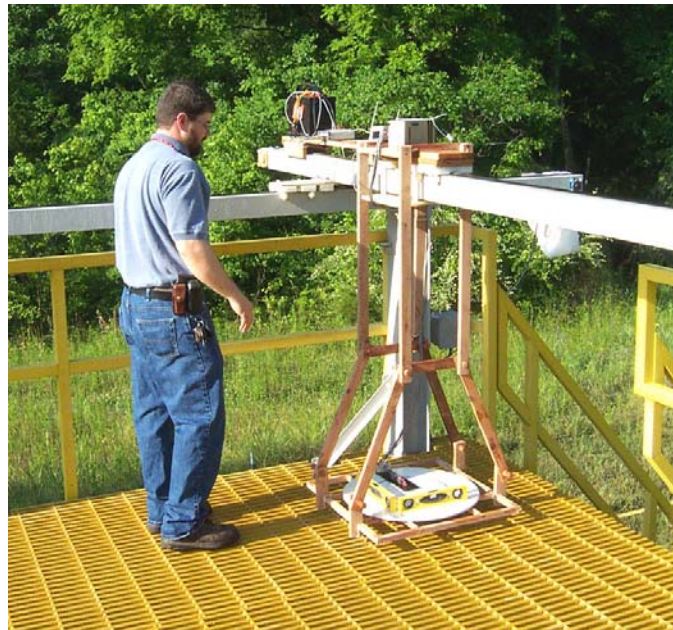
Figure 10. The GEM3 sensor was attached to a carriage on the gantry.
