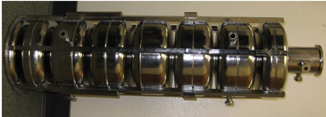
Figure 2. Accelerator cavity of a superconducting linear accelerator.
