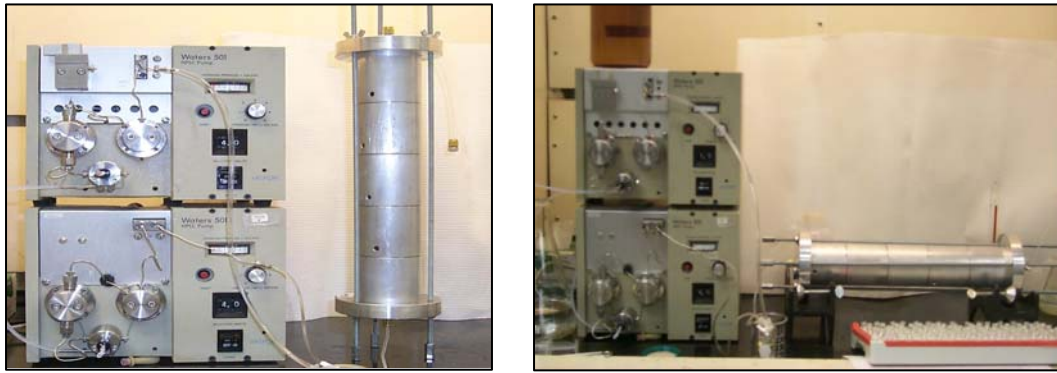
Figure 3.38. Setup for Column Experiments with Surfactants
