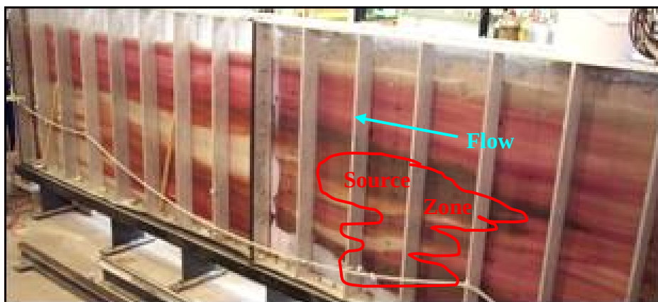
Figure 3.91. Oxidation during ISCO High Heterogeneity Experiment
