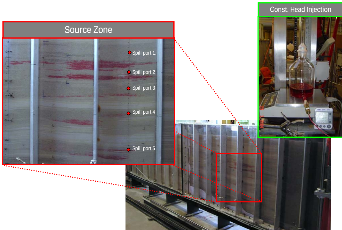
Figure A1.7. Spill device, location, and final NAPL distribution
