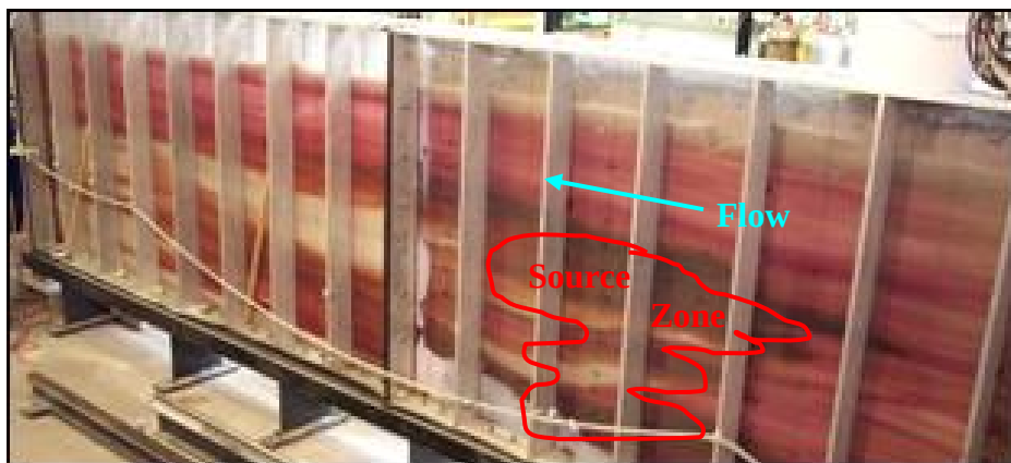
Figure A1.16. Large-Scale Tank during Chemical Oxidation.
