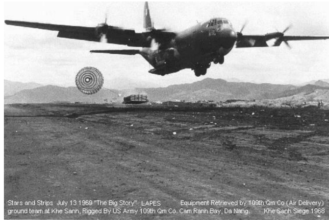
Figure 3. C-130 performing LAPES cargo drop during the siege of Khe Sahn in 1968. (Source: http://www.qmfound.com/khe_sanh1.jpg )
