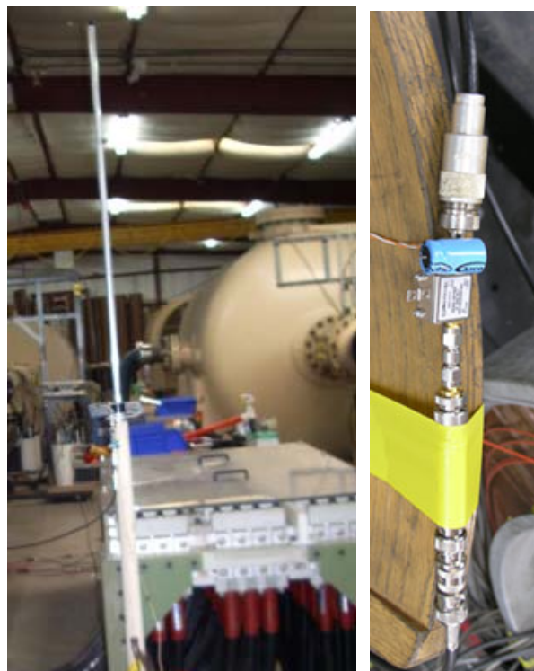
Figure 3. Antenna used to measure broad band RF radiation present during the tests. The signal is directly applied to a 100 MHz high-pass filter and 20 dB broadband amplifier (close-up at the right) before transmission via RG-8 coax to the digital oscilloscope.
