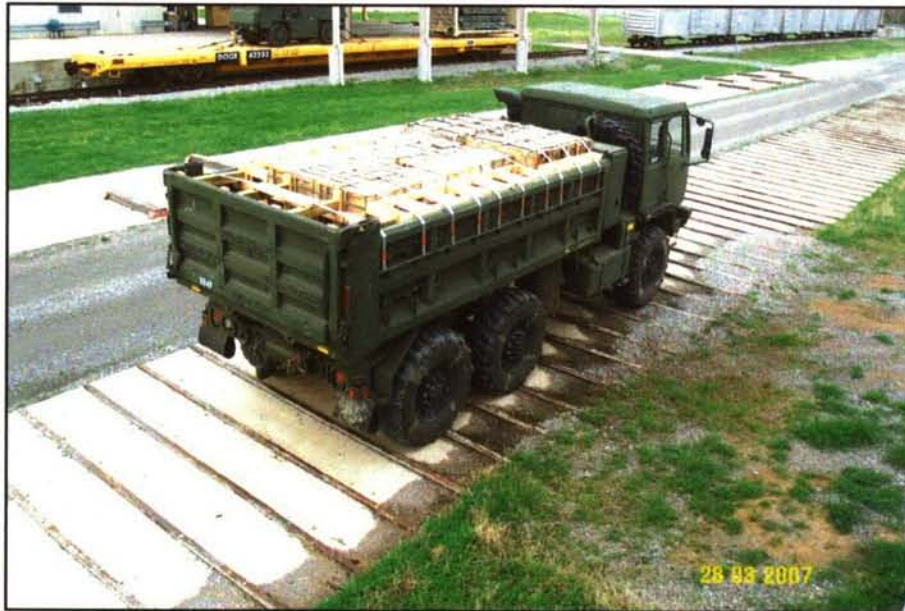
Photo 4. 10-Ton Dump Truck on the Washboard Course
