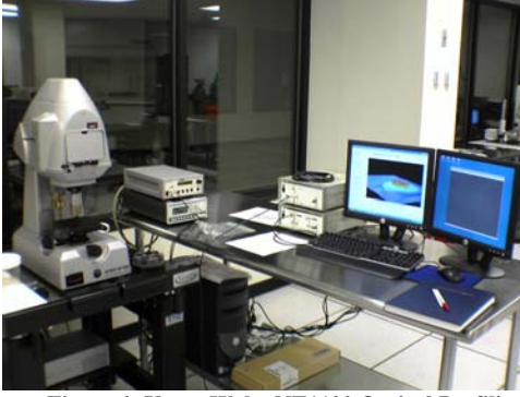
Figure 4: Veeco Wyko NT1100 Optical Profiling system (left), and a MEMS die being probed on this setup for motion characterization.
