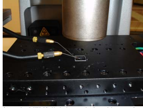
Figure 4: Veeco Wyko NT1100 Optical Profiling system (left), and a MEMS die being probed on this setup for motion characterization.
