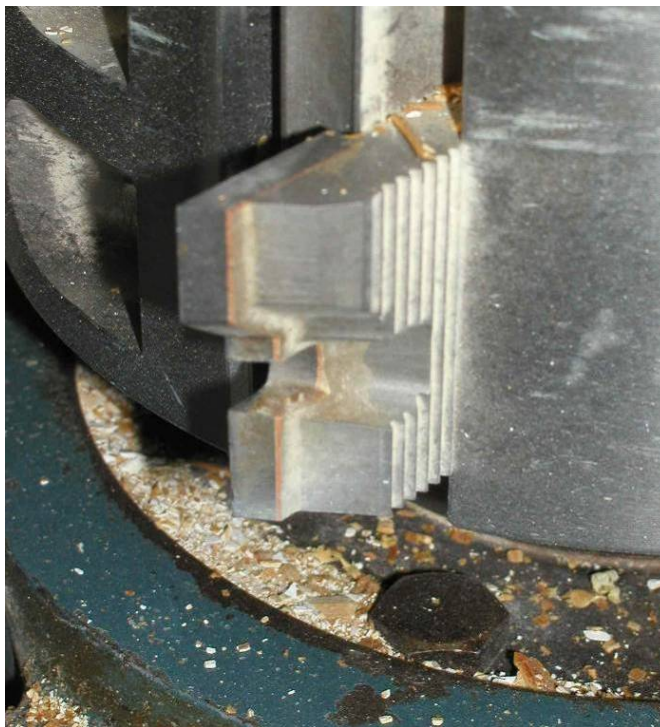
Figure 14. Carbide knife used to machine southern pine, showing corrugation on back.
