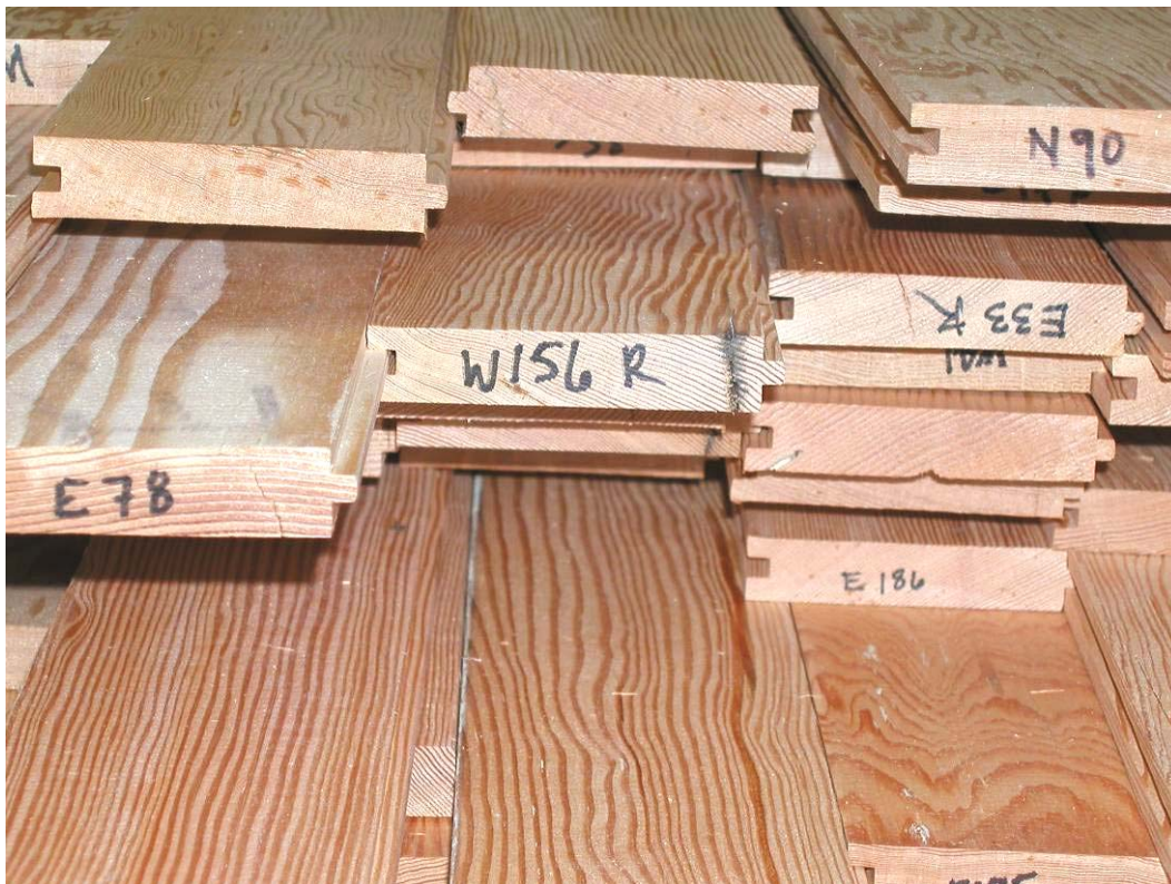
Figure 30. T&G flooring produced from Fort Ord siding.
