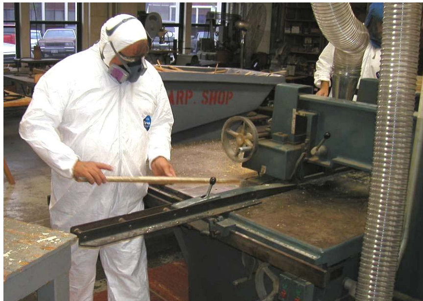
Figure 17. Ripping of siding to width.
