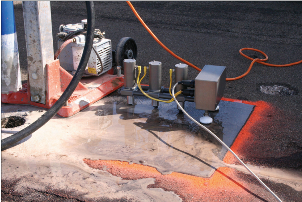
Figure 6. Obtaining the in situ modulus using the PSPA.
