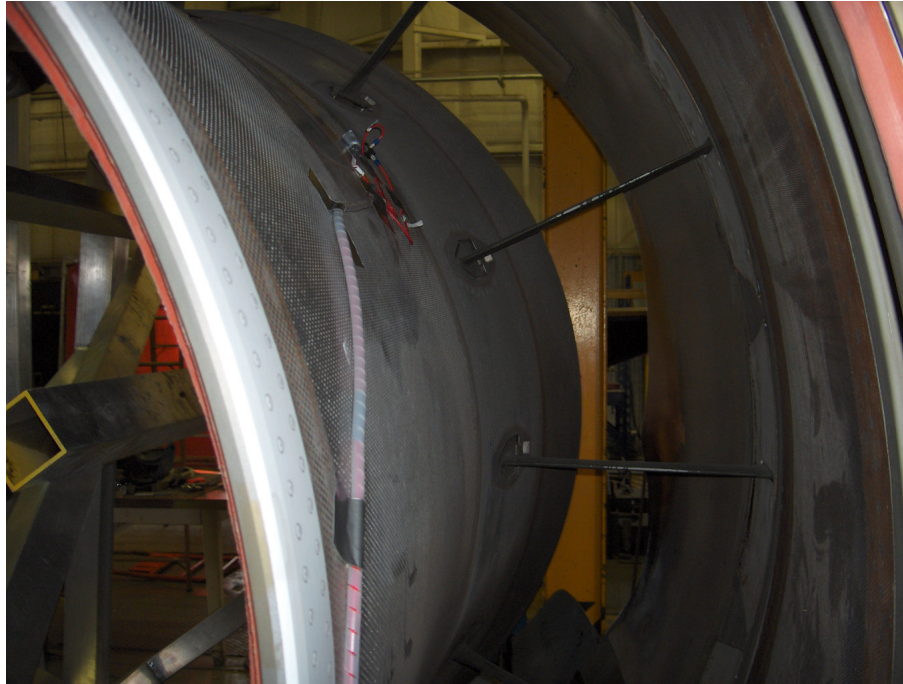
Figure 11. Placement of triaxial accelerometer.
