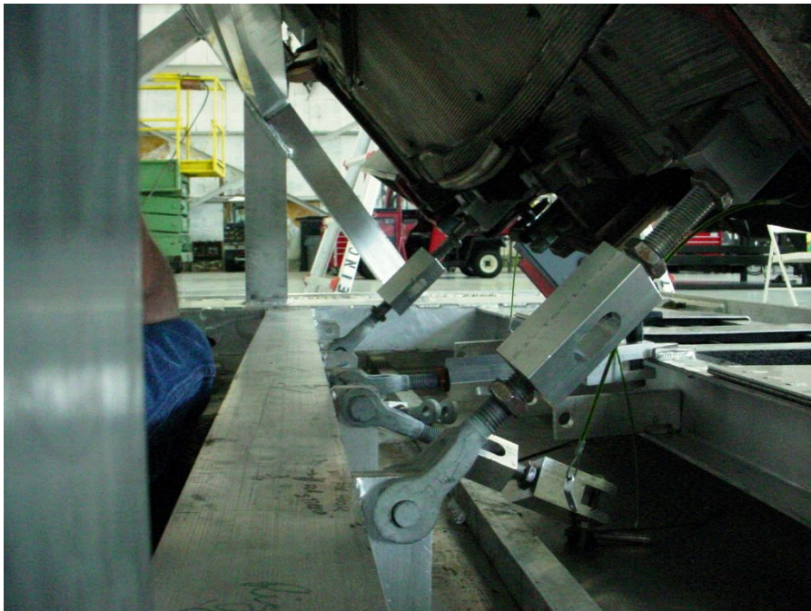
Figure 6. FTR bottom cradle attachment points.
