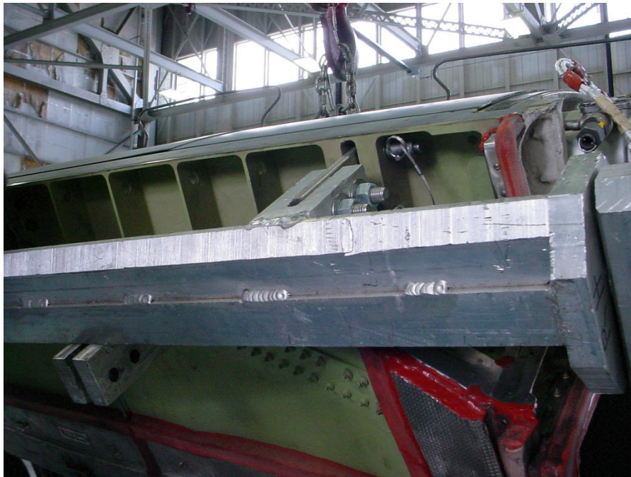
Figure 4. FTR top cradle attachment points.
