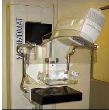
Fig. 1: The prototype multi-projection breast imaging instrument.
