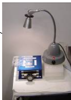
Figure 10. Apparatus employed for illuminating B. anthracis spores upon photosensitizer treated fabric.
