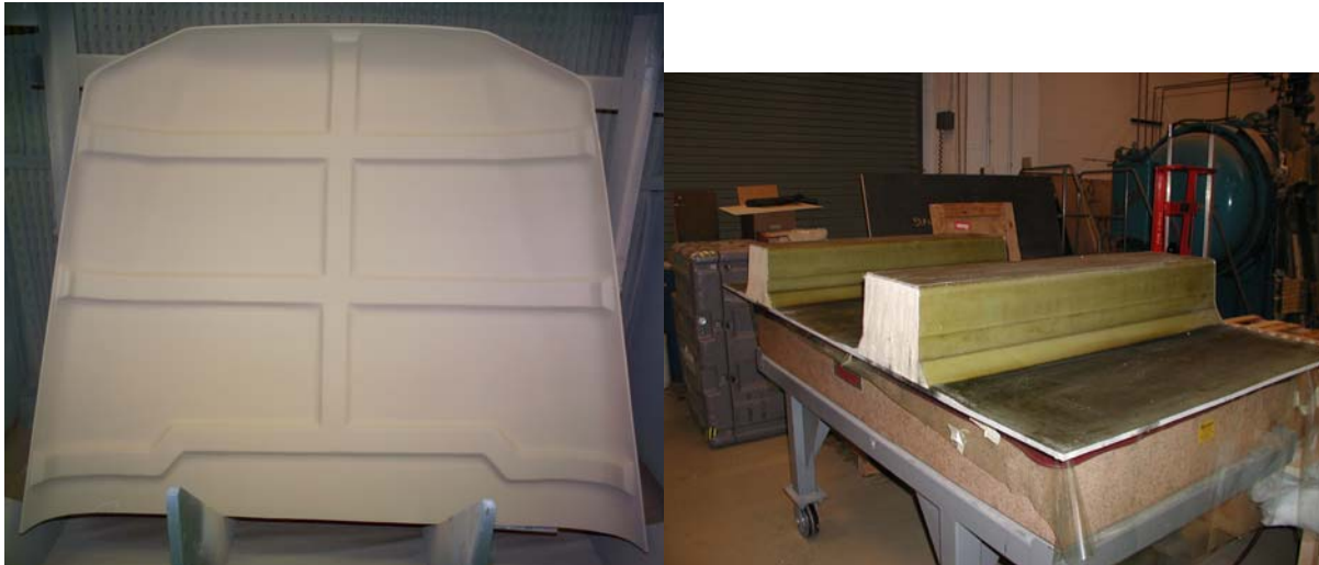
Fig. 7: M35A3 hood (left) and hat stiffened structure (right) for Advanced Sail Program and DDX prepared using FAVE-L resin.
