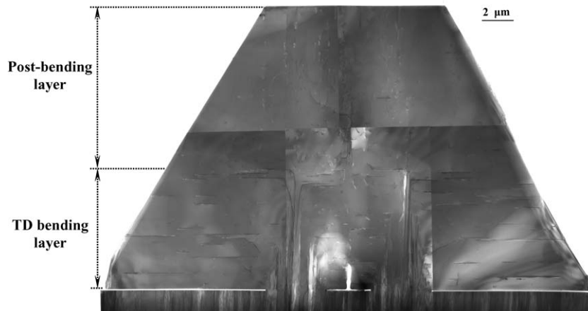
Fig. 5. Bright-field cross-sectional collaged TEM image of modified LEO nonplanar GaN at the end of the second step along the [1\bar{1}00] zone axis.
