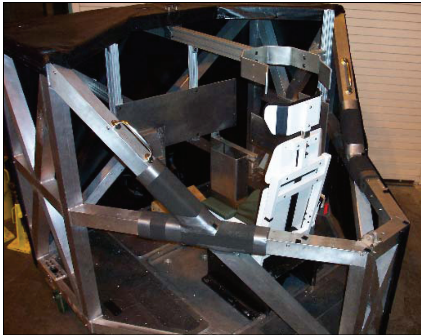
Figure 1. Interior of the RMS, including the aluminum brackets simulating the potential impact points for the head (including the cupola), arms, and legs.
