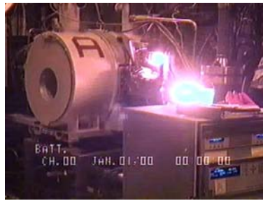
NaK Injection Off – Engine Lit (26.13 s)
