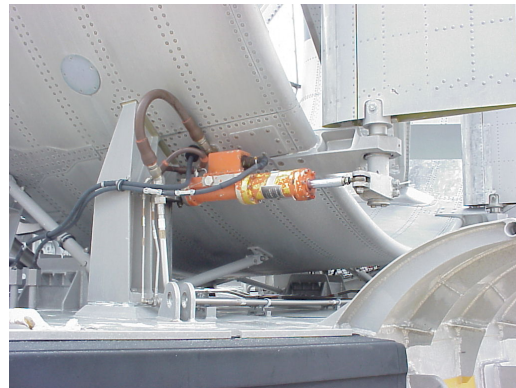
Fig. 1. Conventional hydraulic steering vane control system of the LCAC.
