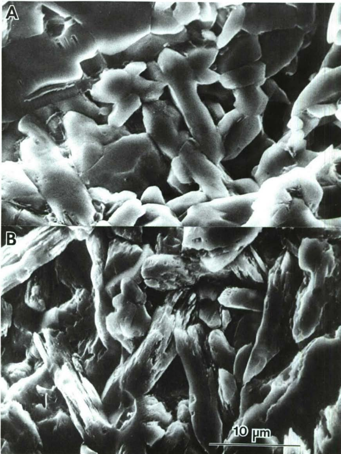
Fig. 2. Sintered SiC specimens reacted with \text{NaCO}_3 at 1000^\circ\text{C} for (A) 1 h and (B) 48 h. Reaction product removed by HF.
