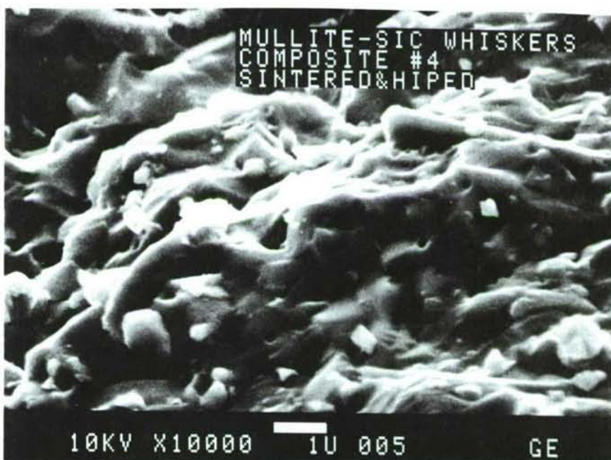
FIGURE 14A FRACTURE SURFACE MULLITE-SiC WHISKER-GLASS I - Al_2O_3 (70/30/20/48 PARTS BY WEIGHT) SPECIMEN NO. L3
