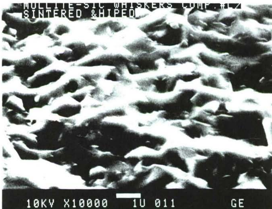
FIGURE 16A FRACTURE SURFACE MULLITE-SiC WHISKER-Nb 2 O 5 (70/30/5 PARTS BY WEIGHT) COMPOSITE NO. L7
