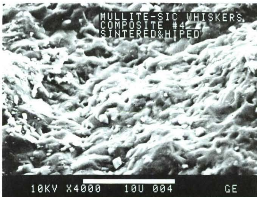
FIGURE 14B FRACTURE SURFACE (SAME AS BELOW)
