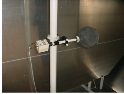
Figure 2.5: E-Field probe on a non-conducting stand in the TEM cell.
