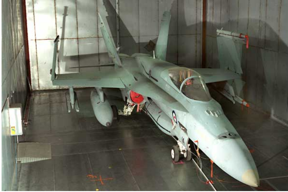
Figure 2.1: DSTO reverberation chamber containing the F/A-18 during the 2001/2002 ASRAAM trial.
