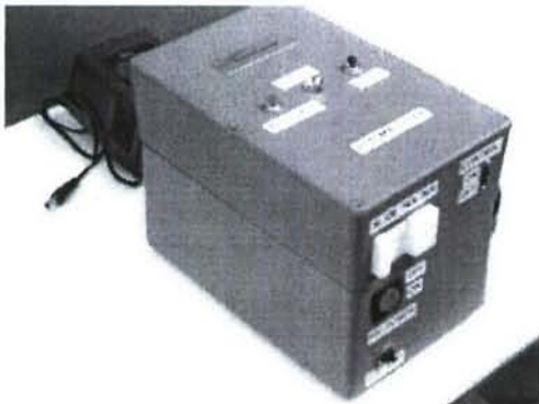
Figure 2. MicroST Plasma Lyser prototype product used for biomaterial extraction and decontamination experiments.
