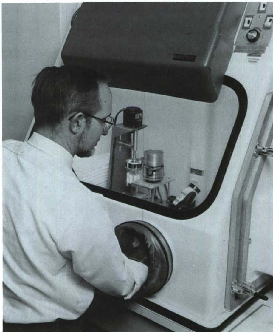
Figure 1. Processing of powder samples in the final riffing stage. The riffing operation is carried out in glovebox which is continuously flushed with dry argon so that samples are exposed to and sealed under an inert atmosphere.
