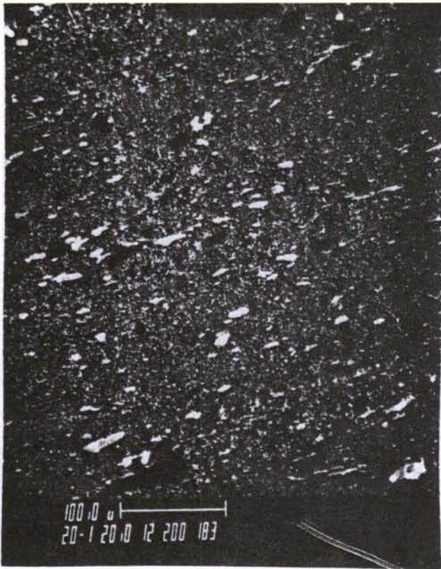
Figure 1. Dense \text{Si}_3\text{N}_4 + 30 v/o \text{ZrO}_2 + 4 w/o \text{Al}_2\text{O}_3 with large \text{Si}_3\text{N}_4 and \text{ZrO}_2 inclusions.
