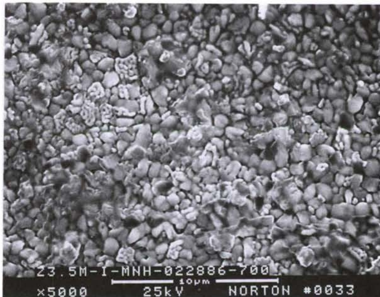
Fig. 2 SEM micrograph (polished and thermally etched surface) of a 1.31 w/o MgO-ZrO 2 ceramic sintered at 1500°C. Powder prepared by ethanol method.
