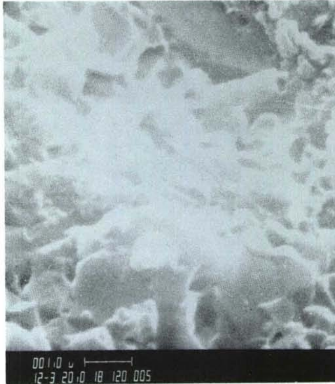
Figure 7. Tateho SCW #1 Flexural Strength Sample Showing No Observed Whisker Pullout or Crack Deflection
