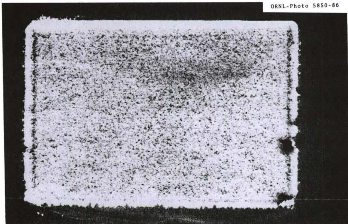
Fig. 2. Ultrasonic scattering data showing detection of 100- \mu\text{m} -diam fiber clumps in a composite ceramic.
