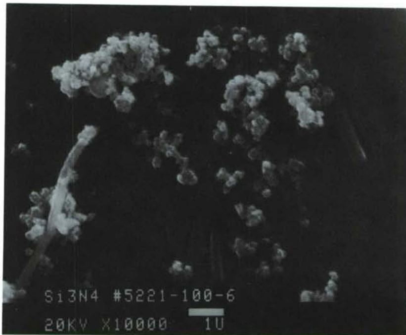
Figure 1. Scanning electron micrograph of powder produced by decomposition of imide synthesized under pressure reaction of \text{SiCl}_4(\text{g}) with \text{NH}_3(\text{l}) .
