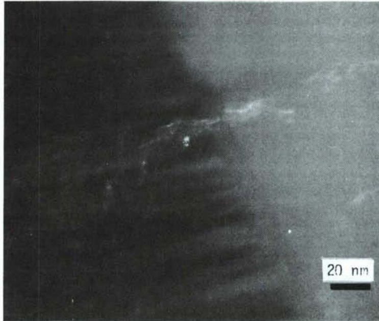
Figure 13. Y-Rich Layer between SiC Whisker and Si 3 N 4 Grain
