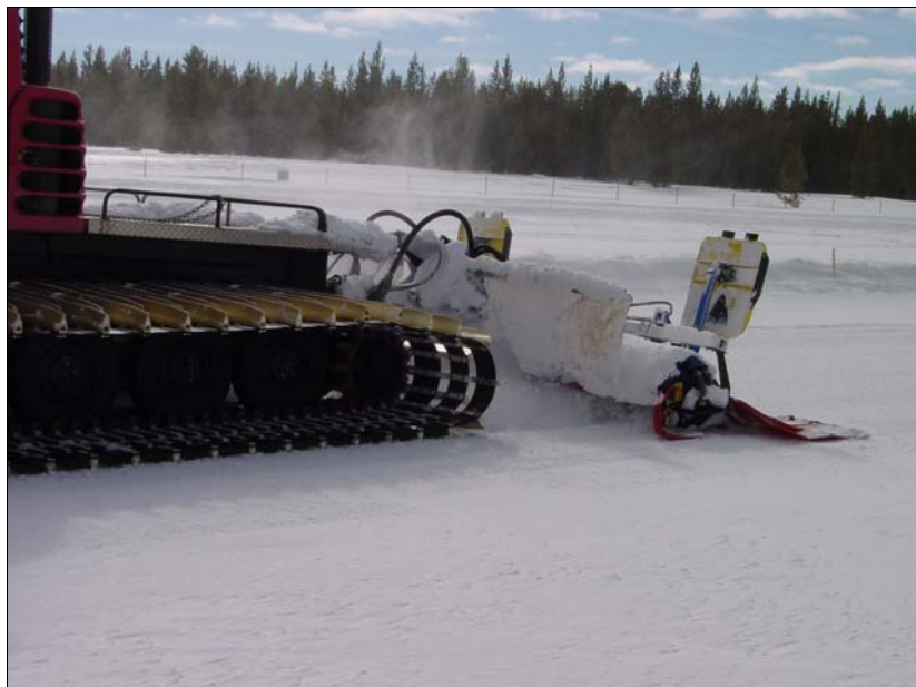
Figure 1. Disaggregating snow with the snow groomer.
