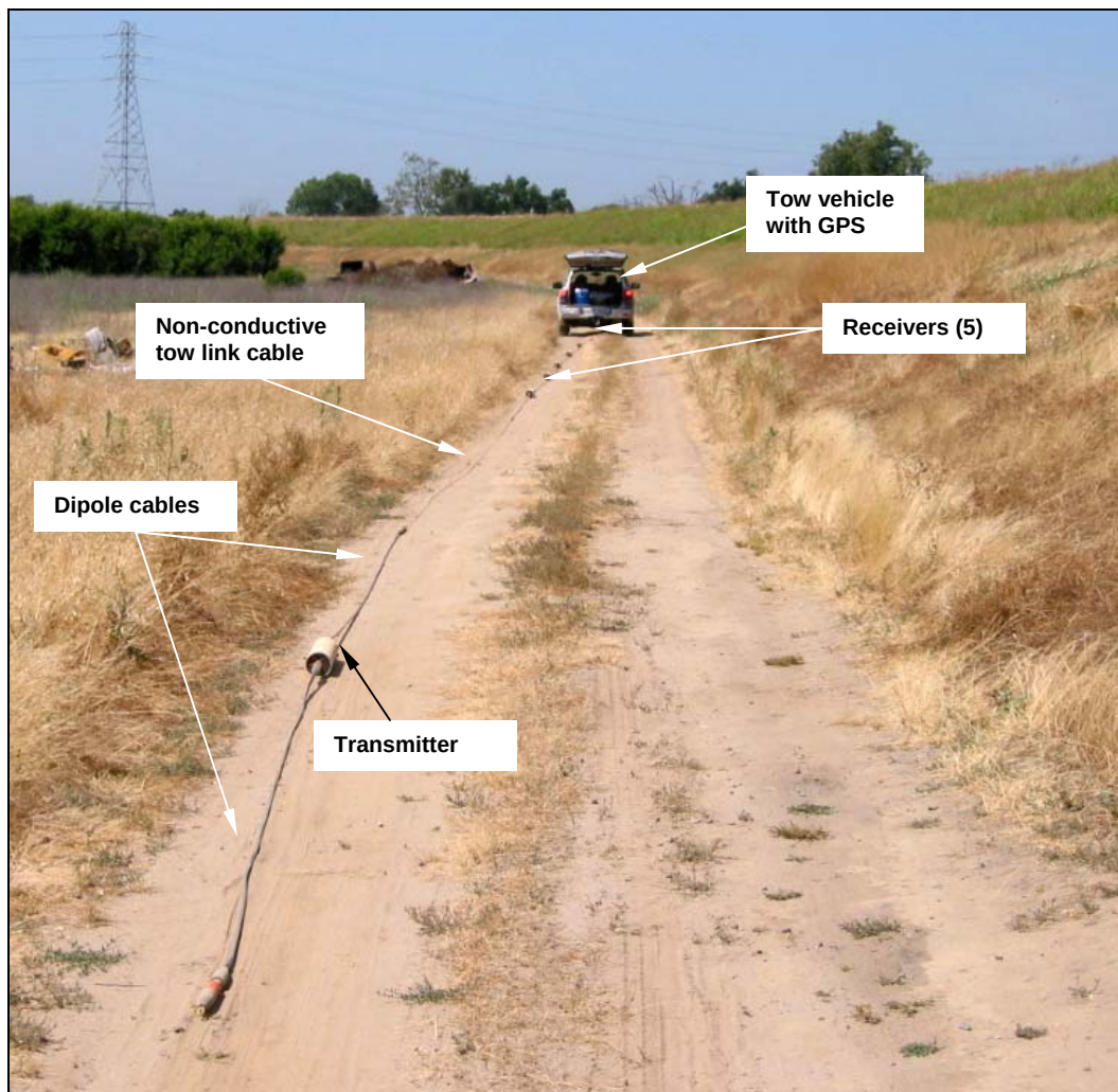
Figure 7. Geometrics OhmMapper capacitively coupled resistivity system being vehicle-towed.
