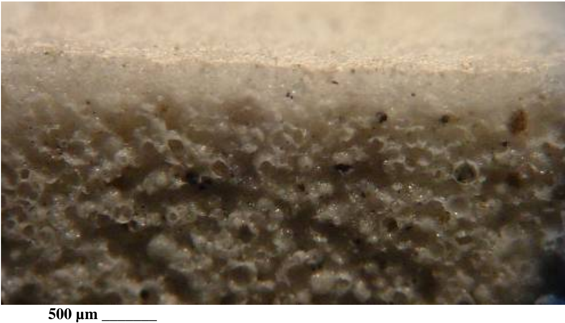
Figure 6: Optical micrograph of coating produced by spray-on with gelling agent on a tooling surface of 2Phase Technologies' reconfigurable tooling material.
