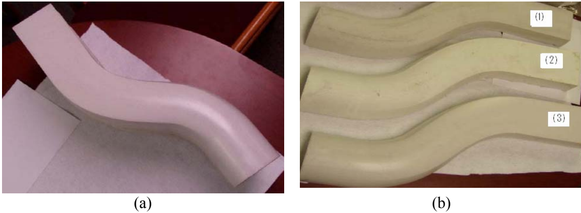
Figure 5: Trapped tooling with coatings: (a) shining surface resulting from tooling with spray-on coating method with gelling agent, and (b) comparison of three finished tools: (1) tool with spray-on coating without gelling agent, (2) tool with brush-on coating and (3) tooling with spray-on coating with gelling agent.
