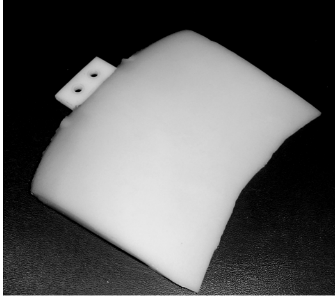
Figure 3.4 Tail fin cut to a size representative of the surface area for the chain pickerel propulsive fins.
