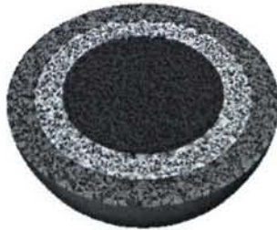
Figure 6: One of the tetrahedral meshes (with 626,561 tetrahedra) used in the computations for the layered sphere.
