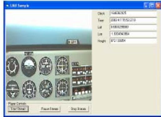
Figure 12: Playback of UAV Encoded Video with Data Extraction
